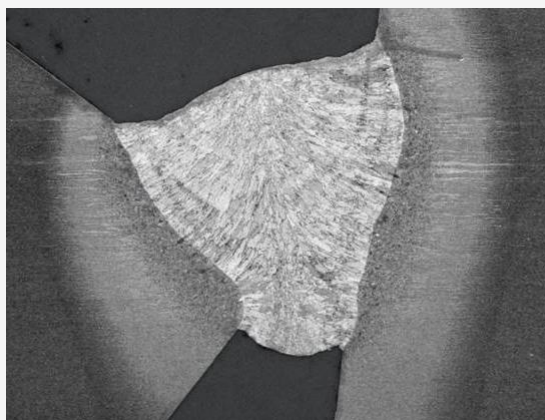
Figure 6.3 A weld repair
